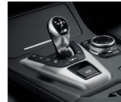
■ Gear lever for the seven-speed M Double Clutch transmission with Drivelogic, with M logo, illumination and M driving dynamics buttons.
