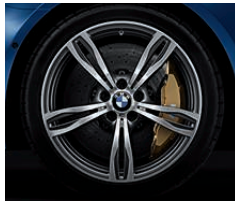
□ 20" M light alloy wheels Double-spoke style 343 M , forged, with mixed tyres. Front: 9 J x 20 with 265/35 R 20 tyres. Rear: 10 J x 20 with 295/30 R 20 tyres.
