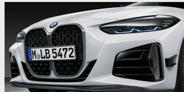
○ Show your style: The frame of the M Performance front grille is made of hand-crafted premium carbon fibre and the decorative slats consist of extra sturdy plastic. A visual highlight at the front of the vehicle for an especially elegant, sporty and individual look.
