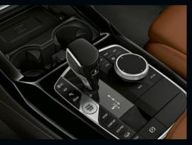
□ The 8-speed Steptronic Sport transmission<sup>3</sup> offers incredibly sporty gear changes. Whether automatic or manual using the selector lever or gearshift paddles – for comfortable coasting or incredibly dynamic driving. In SPORT mode and with the selector lever in the left-hand S/M position, the gear shifts are configured for the maximum performance.
