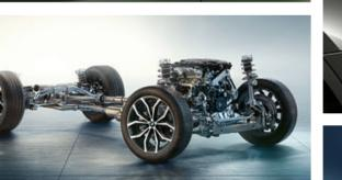
□ The adaptive suspension makes it possible to ideally adjust the damper characteristics to suit any given driving situation, improving roll comfort and driving dynamics. In addition to the standard COMFORT setting for increased driving comfort, the SPORT program can also be selected for athletic damper settings.
